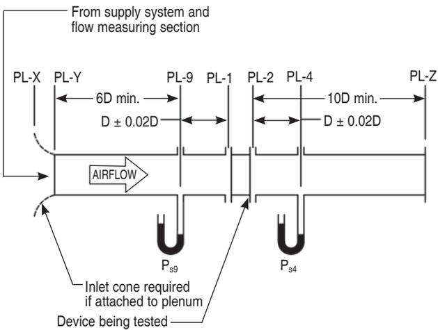
Figure 5.3 - Test Device Setup with Inlet and Outlet Ducts
