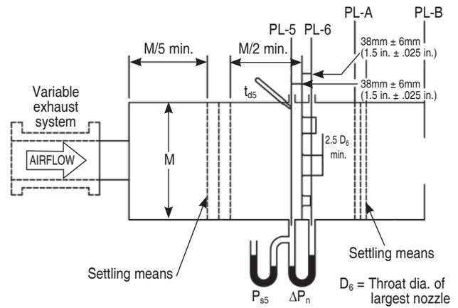
Figure 6.5 - Airflow Rate Measurement Setup - Multiple Nozzle Chamber on Fan Inlet
