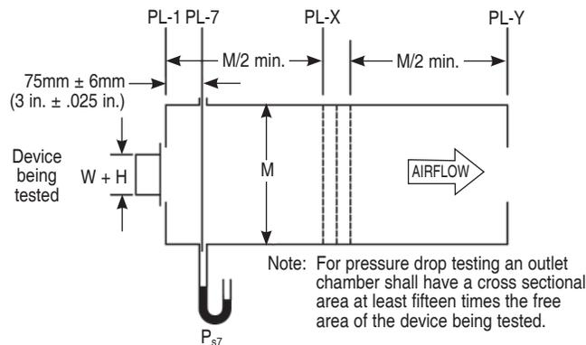
Figure 5.4 - Test Device Setup with Outlet Chamber
