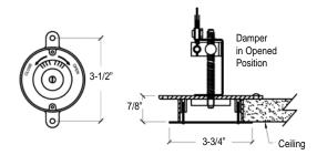
☐ Concealed in ceiling with mtg. bracket Polished Zinc Covered Plate (std.)
