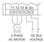
**WARNING** Do not connect incoming AC power to output terminals T1, T2, or T3. Severe damage to the drive will result.
